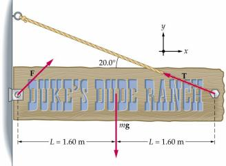
Note that from the sign's point of view the situation is symmetric: it has a movable support at each end and doesn't "know" whether the support is a wall or a wire. So, the force at the wall bolt is the same as it would be if the wall were instead a wire running up and to the right at 20.0° above horizontal. By symmetry, f = T and  $\sum F_y = 2T \sin \theta - mg = 0$ .
